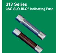
3AG indicating fuses instantly identify themselves upon opening by showing a discoloration of their glass bodies. Guesswork and time consuming circuit testing is eliminated. This unique design offers the same quality performance characteristics as the standard 3AG fuse design.
