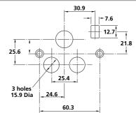
All dimensions in mm. General tolerance ±0.13mm. These dimensions are a guideline only, more detailed drawings are available upon request.
