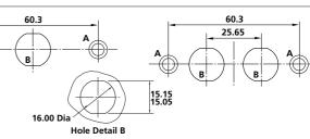
2 holes 3.048mm dia countersunk to 5.08mm dia at 90° (for 6BA screw) and alternatively tap 6BA
