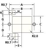
All dimensions in mm. General tolerance ±0.13mm. These dimensions are a guideline only, more detailed drawings are available upon request.
