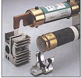
Class R and CC fuse holders have a rejection feature which prevents the mounting of a fuse with lower interrupting capacity. The size of Class T and J fuse holders prevent the mounting of a fuse with lower interrupting capacity.
