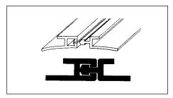
Loc-Trac® provides an effective closure that is ideal for use where the assembly will be subjected to random flexing.
