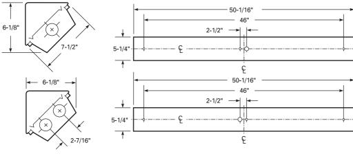
$A=5/16^{\circ}$  dia. hole (6)  $B=7/8^{\circ}$  dia. K.O. Dimensions subject to change without notice.
