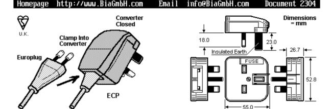
The 2 Pin European VDE Converter Plug (ECP) is an adapter that converts the European CEE VII VDE plug to the BS 1363 system format. The plug is designed and manufactured to meet the requirements of BS 5733. It complies fully with the LDV and Plug and Socket safety regulations. The design of the clamping method ensures the body of the European CEE VII plug is enclosed.
