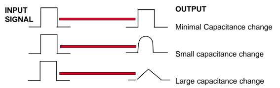
**Capacitance-**The property of a system of conductors and dielectrics that allow the storage of an electrical charge when a potential difference exists between conductors. Capacitance is found between wo wires of a twisted pair, and also between adjacent conductors in the same cable (mutual capaciance). Capacitance is expressed in pf/ft. The larger the capacitance, the higher the distortions.
