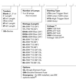
Ballast Type (1) Blank=Standard Magnetic Ballast LE3=T12 Magnetic Energy Saving LEOC8=T8 Magnetic Energy Saving EB8\_= T8 Electronic Instant Start. Total Harmonic Distortion < 20% No. of Ballast
