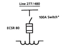
60A Transformer primary Full Load Amperes—Magnetizing current 720 amperes for about 0.1 second.
