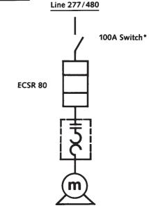
65A Motor Full Load Amperes—Starting current 390 amperes for about 4-8 seconds, normally.
